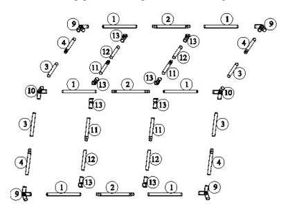
2. Connect the corners and pipes together as shown in the diagram.
