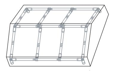
2. Lift the covered frame higher and insert the legs uprights as shown in the diagram.
